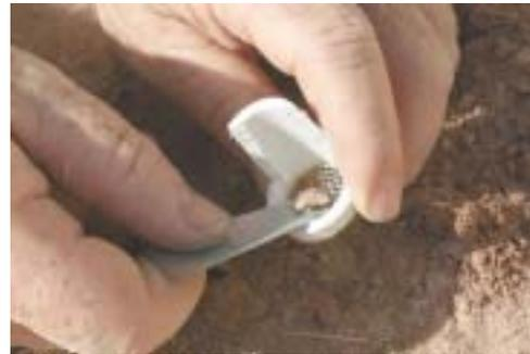
**Figure 16.** Place sample in sieve.
