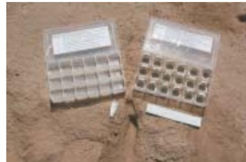
**Figure 19.** Complete soil stability kit with water and samples.
